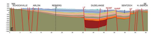
Fig. 6: Regional geological cross sections (horizontal axis in kilometers, vertical axis in meters). Traces of the sections are shown in Fig. 1. The vertical exaggeration is 5-fold for profiles A to E and 7.5-fold for profiles F and G. Black dashed lines correspond to intersection with the indicated cross section.
