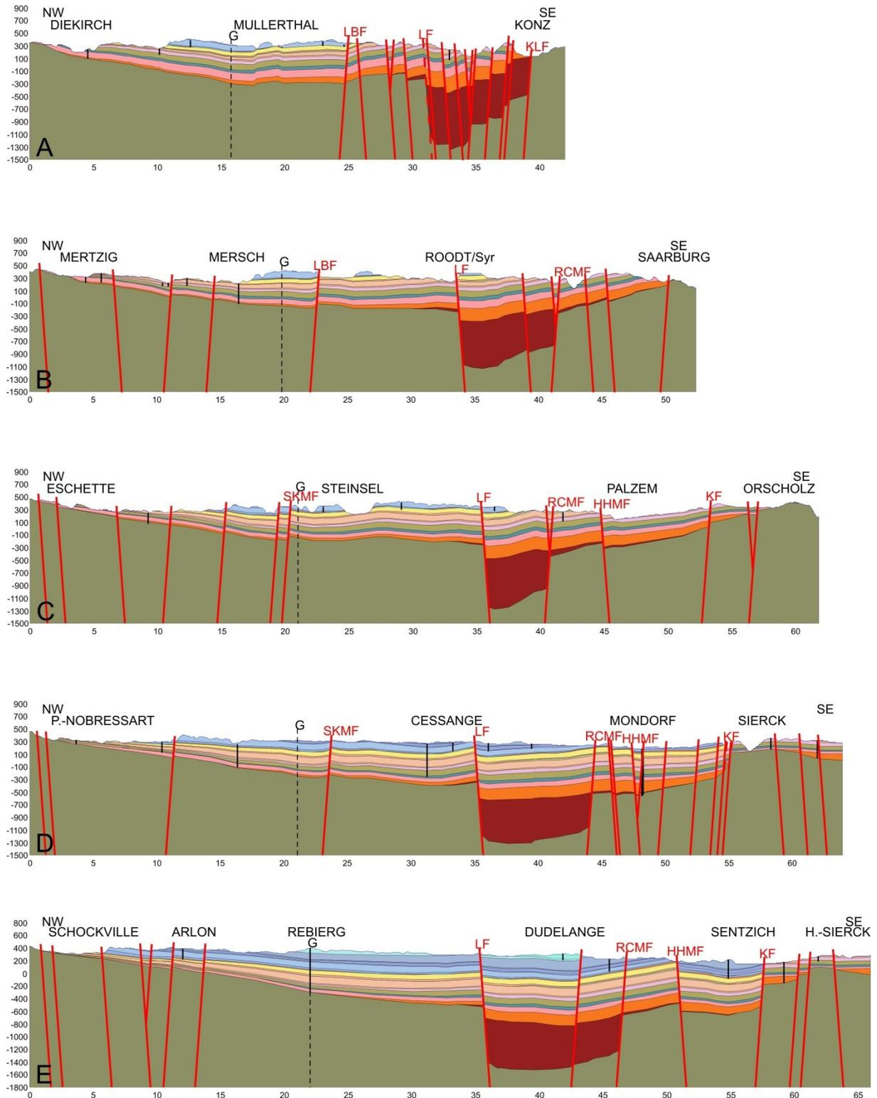
Fig. 6: Regional geological cross sections (horizontal axis in kilometers, vertical axis in meters). Traces of the sections are shown in Fig. 1. The vertical exaggeration is 5-fold for profiles A to E and 7.5-fold for profiles F and G. Black dashed lines correspond to intersection with the indicated cross section.
